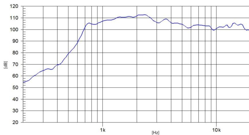
Note: On axis frequency response measured coupled to MA 15 horn in anechoic chamber 1W @ 1m.
