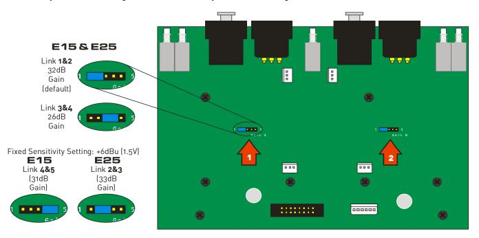
Remember, setting higher gain does not change the maximum available power but changes the level of signal input to achieve maximum power. In any case, provided that the input signal is less than 20dBu/7.7V, the built in limiter circuit will prevent distortion within the amplifier.
