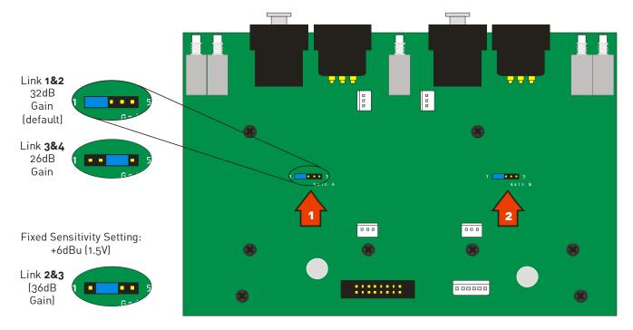
Remember, setting higher gain does not change the maximum available power but changes the level of signal input to achieve maximum power. In any case, provided that the input signal is less than 20dBu/7.7V, the built in limiter circuit will prevent distortion within the amplifier.
