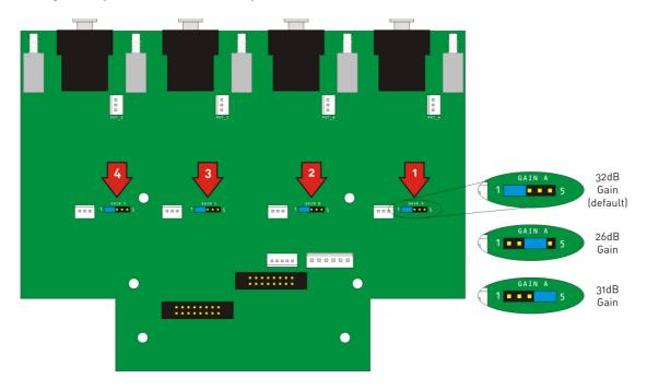
Remember, setting higher gain does not change the maximum available power but changes the level of signal input to achieve maximum power. In any case, provided that the input signal is less than 20dBu/7.7V, the built-in limiter circuit will prevent distortion within the amplifier.
