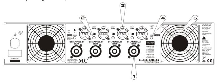
1: Channel A output Speakon socket: Normal output is on pins 1+ hot, 1- cold. Channel B's output is also wired to this socket to enable a single NL4 to provide both channels and to facilitate easier wiring in bridged mode. Channel B is wired pins 2+ hot, 2- cold.
