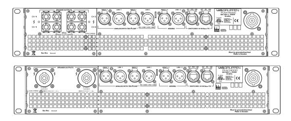
**The PLM 14000** is available with either binding posts or an "embedded patch panel" with Neutrik speakON connectors (2 x NLT4). Common connectors include; 2 x analog input XLR with switchable Iso-Float, 2 channels of AES/EBU with link-through capability for daisy chaining, 2 x EtherCON® for linking or redundancy. A 32 amp PowerCON® connector is used for mains supply.
