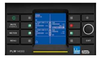
**The front panel** is the "local control center" for the PLM 14000. An intuitive, menu driven interface allows quick access to key functions using the moisture resistant silicone touchpad. Information is clearly displayed on the daylight-readable, 2.5-inch LCD panel. The soft-button keypad and precision rotary encoder provide control of processing and amplification functions, with key lock available.
